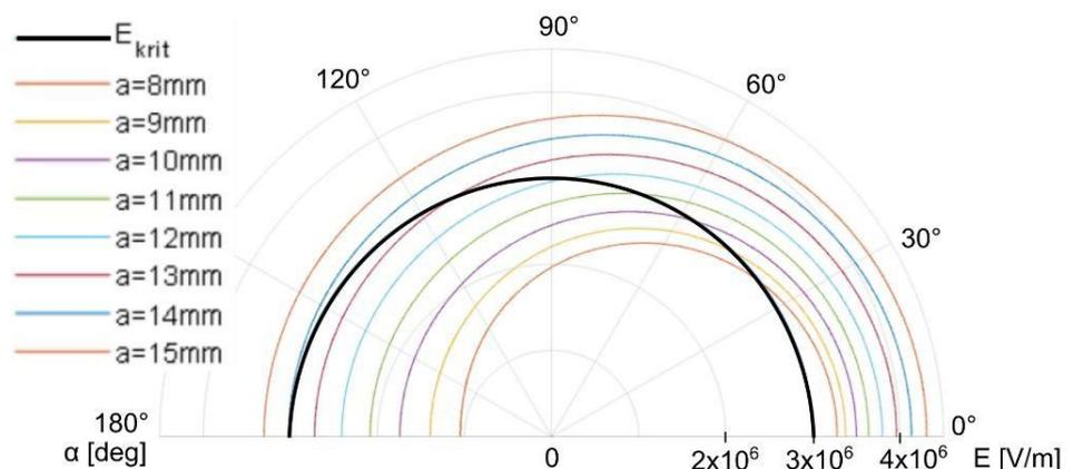
**Figure 4** Electric field strength on the electrode surface as a function of the alpha angle according to Fig. 2.A for selected variants. The black line shows the critical electric field strength.
