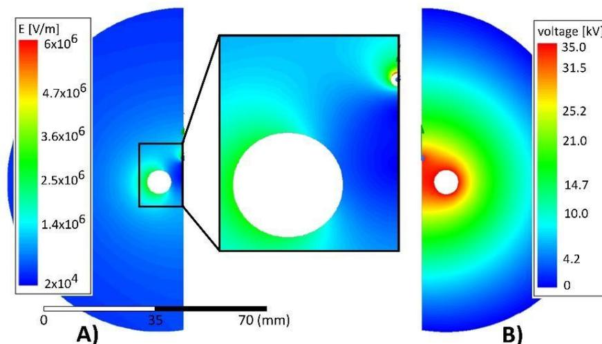
**Figure 3** Distribution of electric field strength (A) and voltage (B) around the electrode with shielding elements according to Fig. 2.A. Applied effective voltage is 35 kV.
