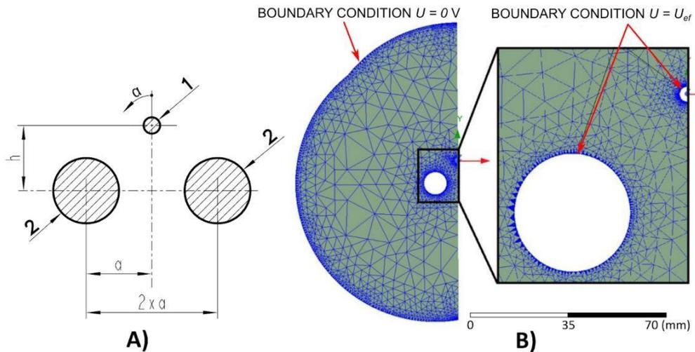
**Figure 2 A:** Schematic representation of cable electrode (1) with shielding elements (2) in section. **B:** Model of the air environment around the electrode, the shielding elements and the virtual collector with the maximum mesh size: near the electrode - 0.001 mm, near the shielding elements - 0.01 mm.
