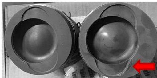
Figure 2 Comparison of correctly (left piston) and incorrectly (right piston) made valve selection in the piston
