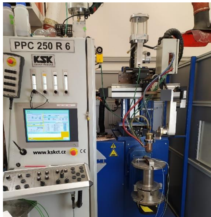
Figure 1 Plasma hardfacing automate PPC 250 R6, KSK, Ltd.
