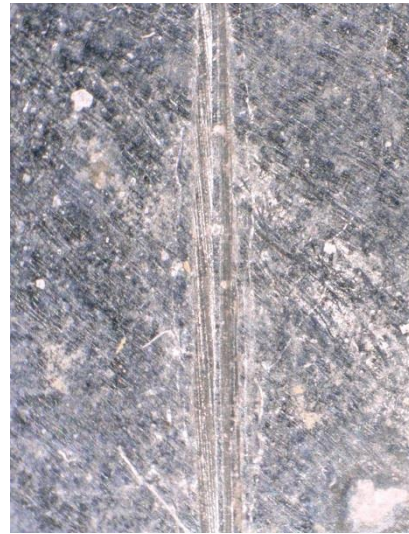
Figure 6 Detail of the scribe on the weld metal, 50x magnification Figure 7 Detail of the scribe on the base material, 50x magnification
