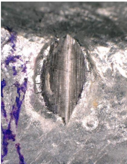
Figure 6 Detail of the scribe on the weld metal, 50x magnification Figure 7 Detail of the scribe on the base material, 50x magnification
