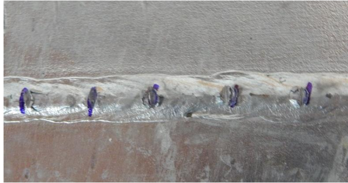
Figure 5 Photograph of the sample after the adhesion test on the weld.
