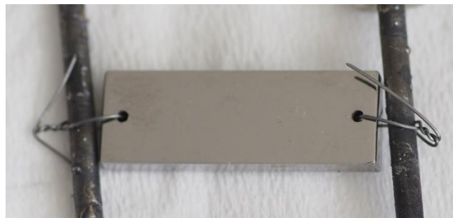
Figure 1 Sample of Inconel 625 alloy in the holder before exposure
