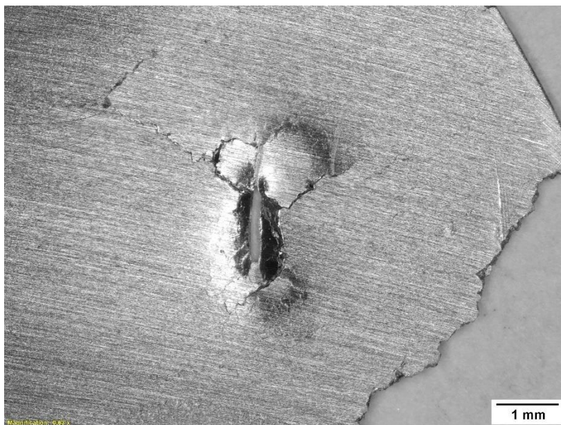
Figure 2 The degradation caused by tin pest
