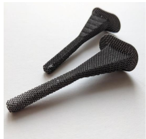
Figure 8 Implants printed from the recycled TiNbTaSn alloy
