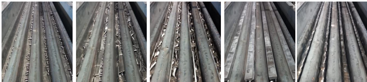
Figure 2 The method of distributing the input material to the H-PAM copper crystallizer.
