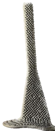
Figure 8 Implants printed from the recycled TiNbTaSn alloy
