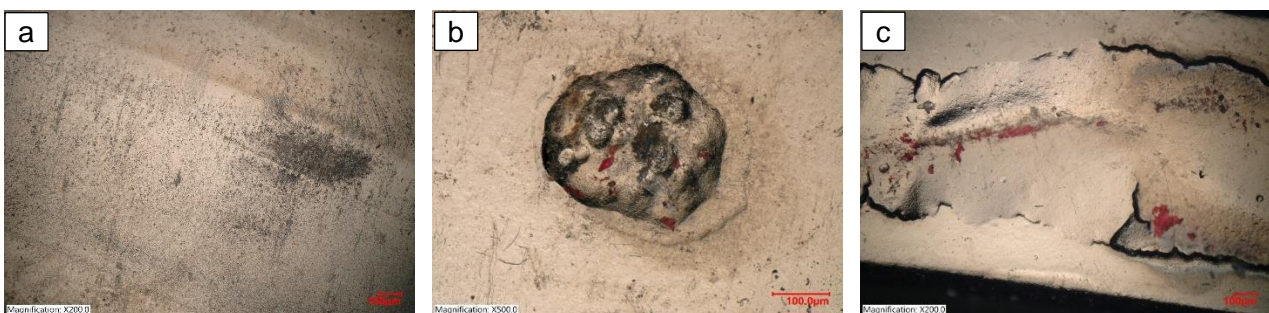
Figure 4 Examples of defects on NiDi coating (sample B)
