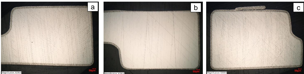
Figure 5 Examples of NiDi coating cross sections
