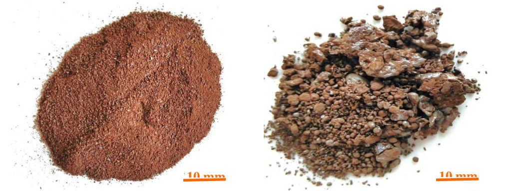
Figure 4 Fine fraction (left), metallic part (right)
