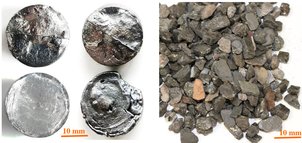
Figure 3 Castings of secondary lead (left), coarse fraction (right)
