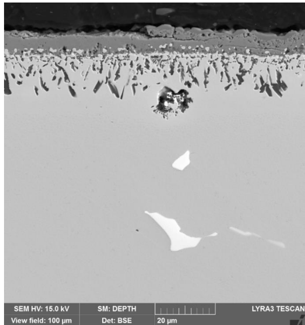
Figure 4 SEM BSE image of specimen exposure at 750 °C for 1000 h
