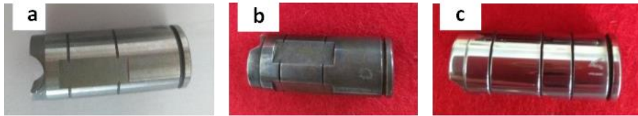
Figure 3 The surface of 16MnCrS5 steel samples: a) initial state after fine grinding, b) after first stage (reduced roughness), c) after second stage (mirror gloss)
