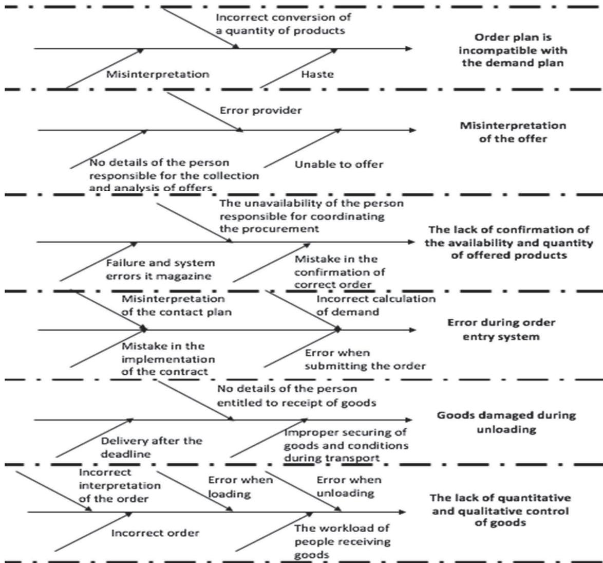
Figure 2 Ishikawa diagrams for potential defects
