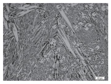
Figure 2 Structure of coating made with string bead, magnification x500
