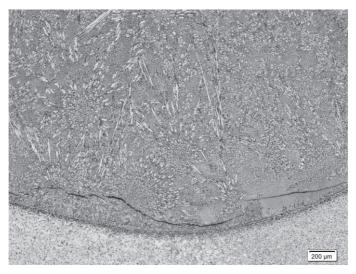
Figure 1 Structure of coating made with string bead, magnification x50
