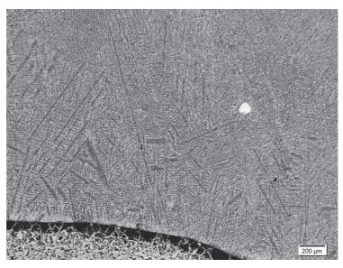
Figure 3 Structure of coating made with weave bead, magnification x50
