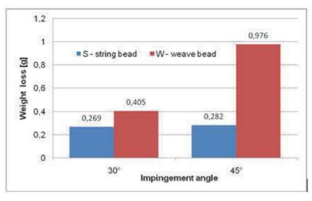
Figure 6 Results of erosion tests
