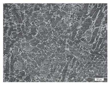
Figure 4 Structure of coating made with weave bead, a) magnification x50, b) magnification x500
