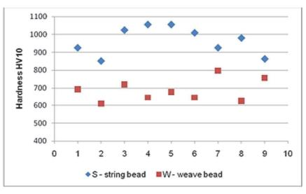
Figure 5 Hardness distributions in hard facing
