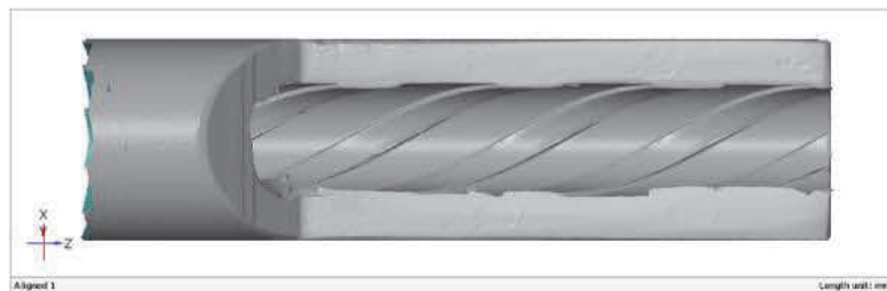
Figure 2 Optical 3D scan of multi rifled tube
