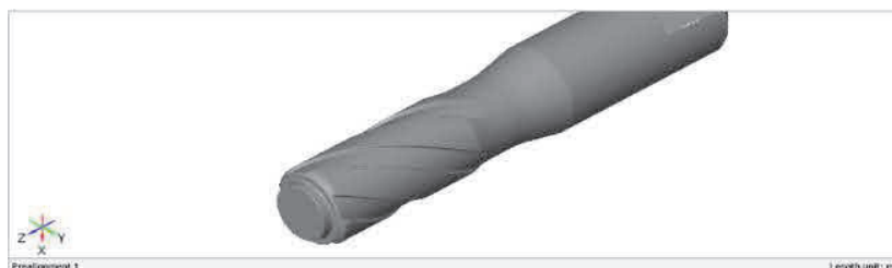
Figure 3 Optical 3D scan of multi rifled plug
