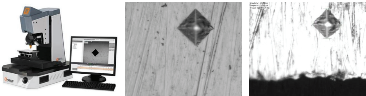
Figure 5 Measurement of micro-hardness by Vickers: Qness Q30A (left) and examples of impressions (right)
