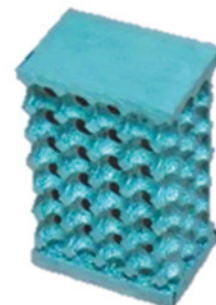
Fig. 5 The sample for the pressure test
