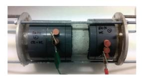
Fig. 2 Experimental design of accelerated migration tests
