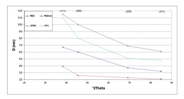
**Fig. 4** Crystallite size of the material Cu 5 vol.% MgO material after various stages of preparation for the plane (111), (200), (220) and (311)
