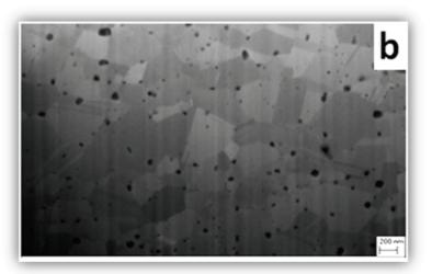
Fig. 1 Microstructure of the Cu-MgO material: (a) light microscopy (b) SEM prepared by FIB
