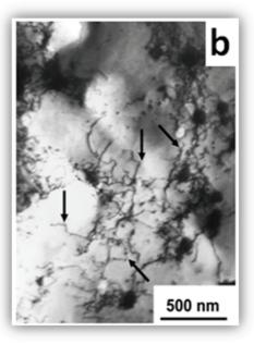
**Fig. 2** The microstructure of the material Cu-3 vol.% MgO material by TEM: (a) detailed view, (b) the interaction of particles with dislocation
