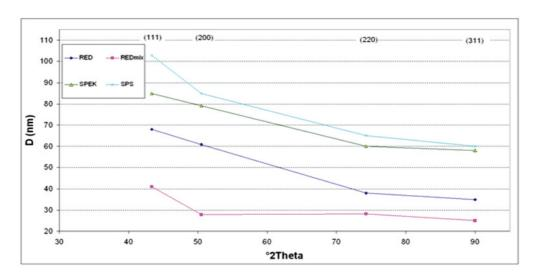
**Fig. 3** Crystallite size of the material Cu 3 vol.% MgO material after various stages of preparation for the plane (111), (200), (220) and (311)
