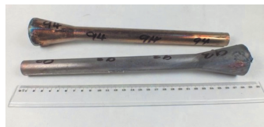
Fig. 2 Experimental alloys after VIM a centrifugal casting
