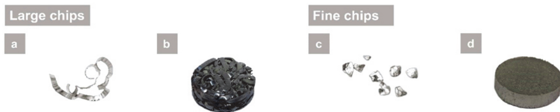
Fig. 1 Initial morphology of as machined and as compressed billets of (a, b) large and (c, d) fine chips
