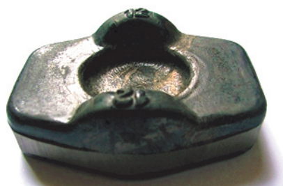
Fig. 8 P/M FeAl alloy part forged at 900 °C
