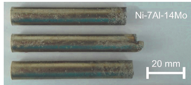
Fig. 1b Castings of the Ni-7Al-14Mo (wt.%) alloy prepared by an induction melting
