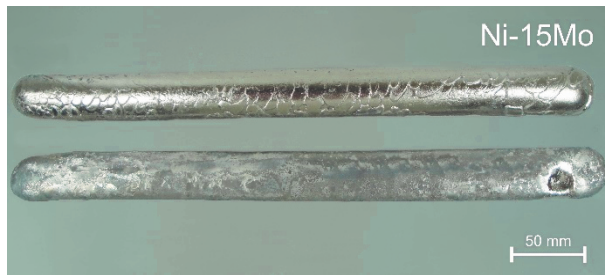
Fig. 1a Ingots of the Ni-15Mo (wt.%) master alloy prepared by a plasma metallurgy
