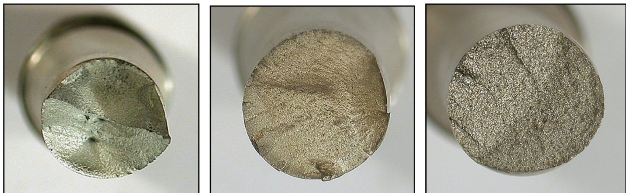
Fig. 6 Morphology of fatigue fractures: aluminium alloy 2017A (left), magnesium alloy AZ31, titanium alloy Ti-6Al-4V (right)
