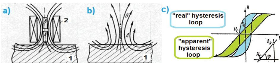
**Fig. 1** Magnetic spot - pole method; a) magnetizing; b) measurement; c) linearization of the hysteresis loop in the second quadrant; A, B - Hall sensors; 1 - ferromagnetic material; 2 - magnetizing coil. [8]
