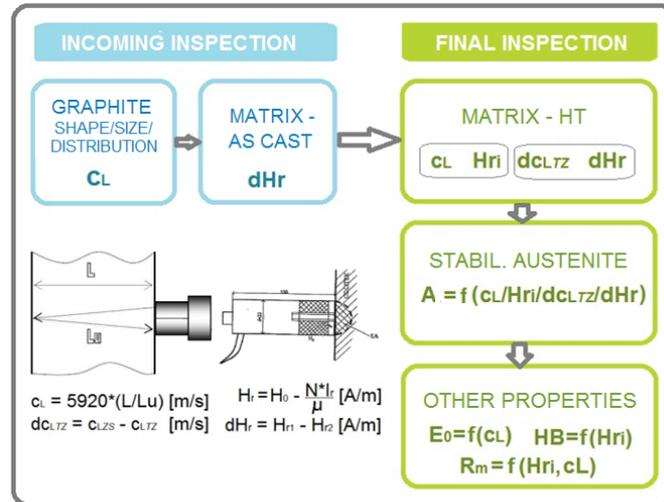
Fig. 4 Diagram of the inspection using ultrasonic speed and residual magnetization.
