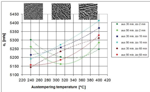
**Fig. 2** The dependence of  $c_L$  on HT conditions (AVGI)
