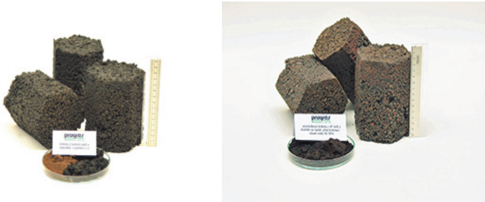
Fig. 2 Practical output of the serial production ProgresEkotech company, s.r.o: 2 a) Briquette from metallurgical metalline dust 2 b) Briquette from blast furnace sludge [13]
