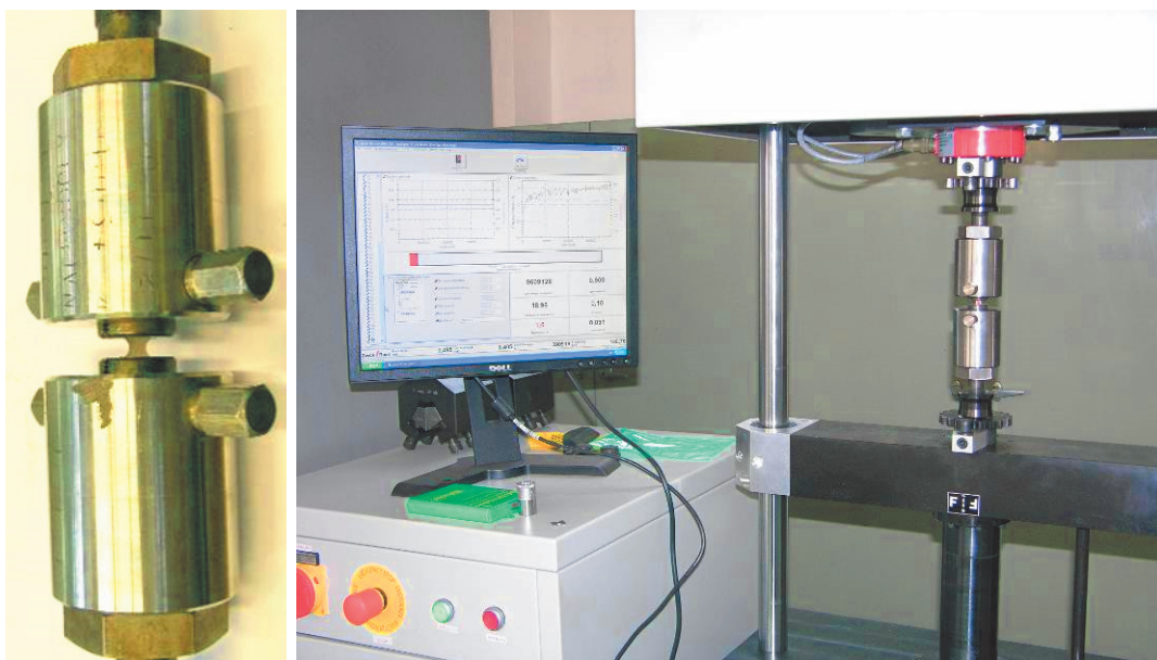
Fig. 6 Principle of fitting SFT specimens (special grips)
