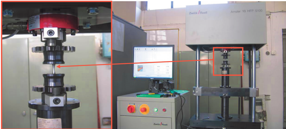
Fig. 5 Testing machine Amsler 10 HFP 5100. Detail of the standard specimen fitting (left)
