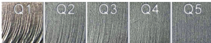
Fig. 5 Water cutting precision class. Q1 separational cut, Q2 through cut, Q3 clean cut, Q4 good edge finish, Q5 excellend edge finish
