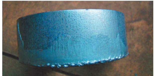
Fig. 3 The edge of metal sheet after cutting with oxygen (Hybrid 200)
