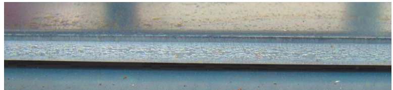
Fig. 4 The edge of the metal sheet after cutting on the guillotine (Durma 3016)
