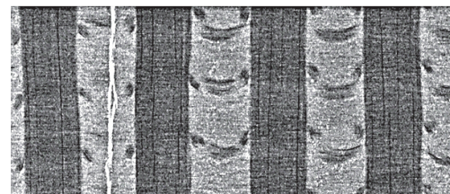
Fig. 3 Computed tomography scan of MMC with embedded optical fibres
