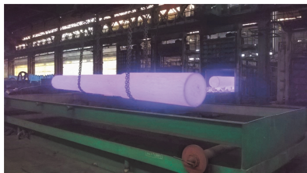
Fig. 4 Quenching of the 42CrMo4 steel
