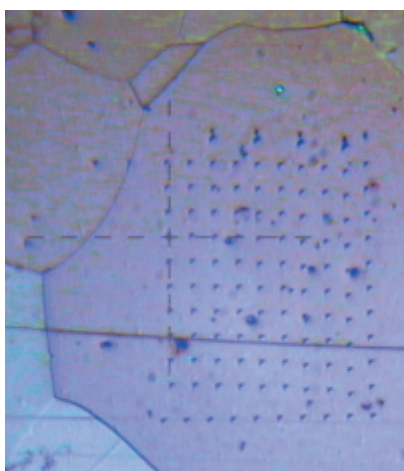
Fig. 3 The indentation array at G3 after room and elevated temperatures measurements
