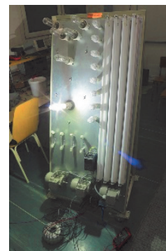
Fig. 10 Special testing board with various types of loads including HID lamps, fluorescent tubes, halogen lamps and electric motors
