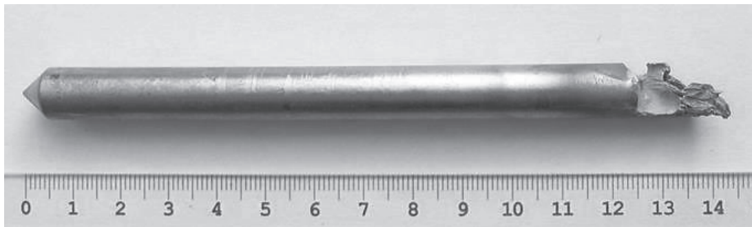
Fig. 1 Rod made from Ni 3 Al alloy after directional solidification
