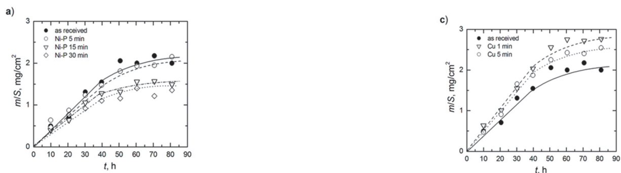
Fig. 2 Mass gain as a function of time during exposure of Nd 12 Co 5 Fe 77 B 6 epoxy resin bonded magnetic material in industrial atmosphere; powder biencapsulated with: a) Ni-P/epoxy resin, b) phosphate/epoxy resin, c) Cu/epoxy resin
