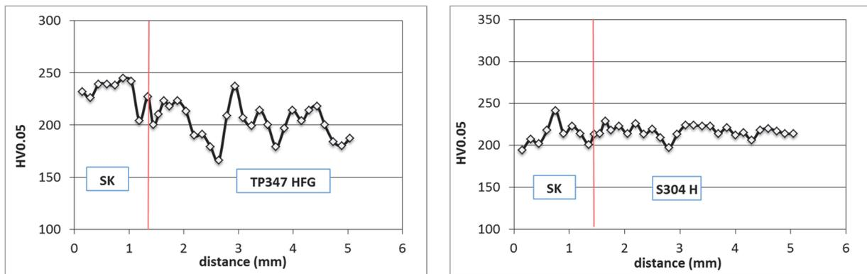
**Fig. 1** Micro hardness profile of heterogeneous weld joint of Tp347 HFG and Super 304H steels after postweld heat treatment
