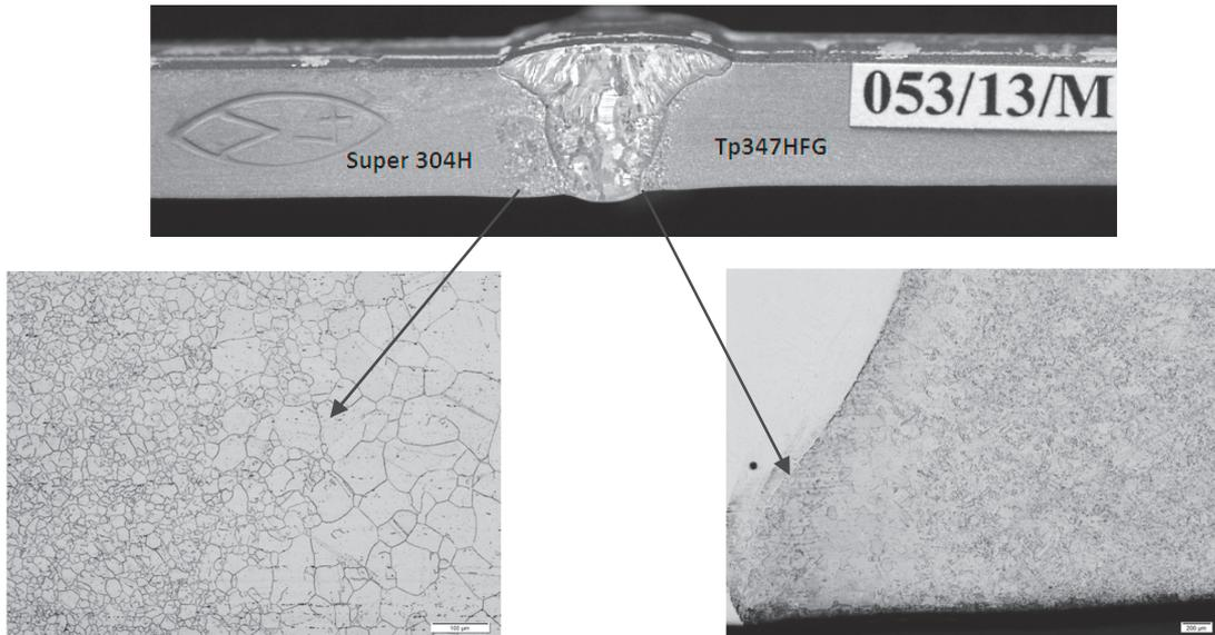
**Fig. 2** Heterogeneous weld joint of Tp347 HFG and Super 304H steels after PWHT including detailed view of HAZ with coarsened austenite grains on both sides of the joint
