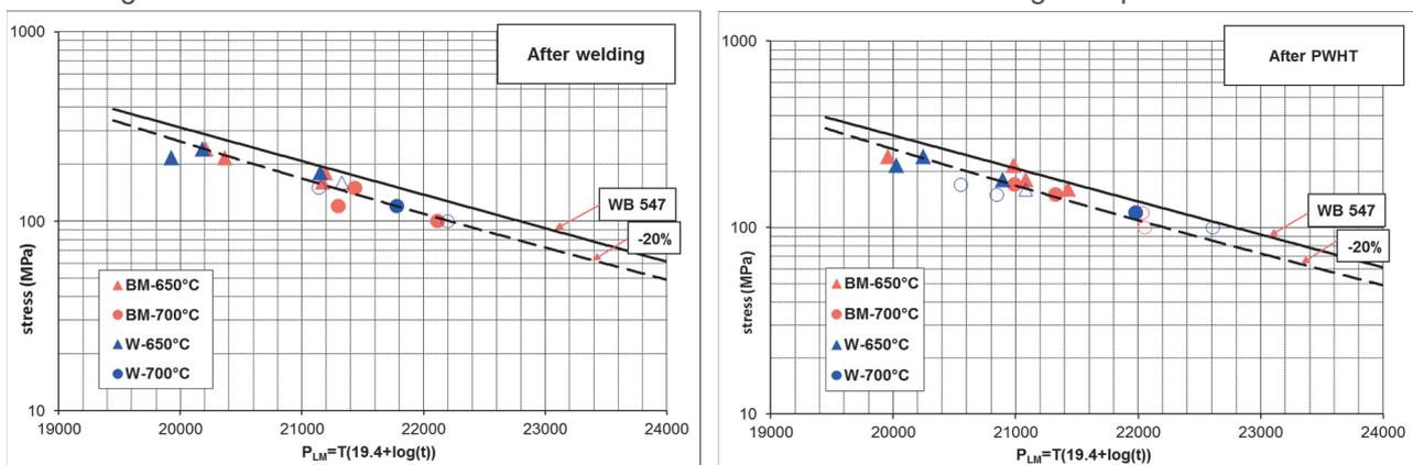
**Fig. 3** Stress dependence of creep rupture strength of basic material and weld joint of steel Tp47 HFG tested on welds with and without PWHT
