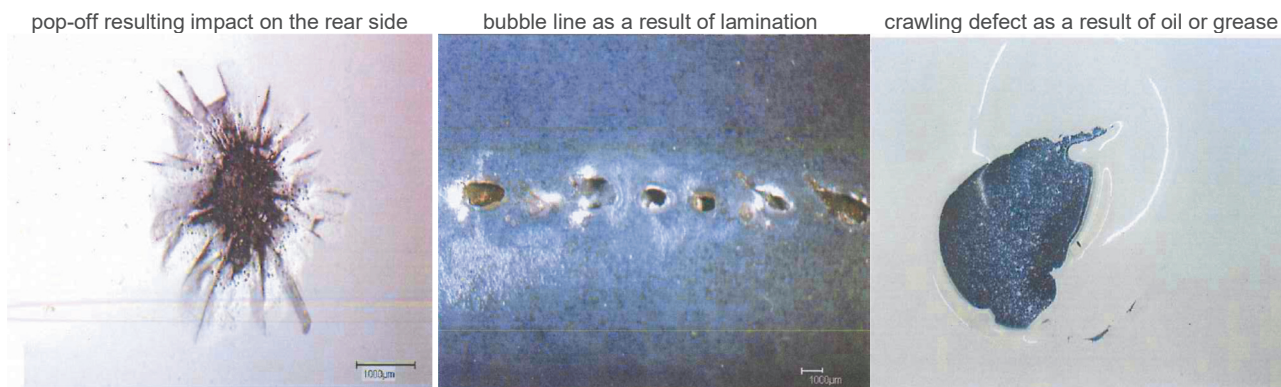
Fig. 2 Example of defects
