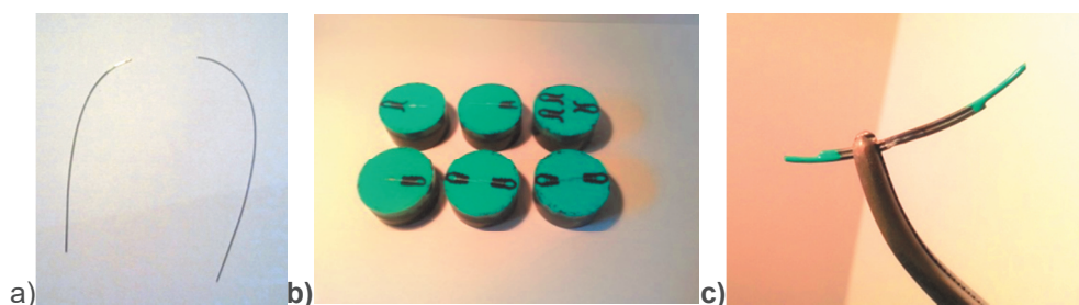
Fig.1 The appearance of tested samples: a) damaged orthodontic arch, b) hot mounted samples of repaired NiTi, c) sample for corrosion test
