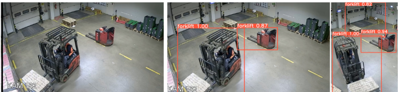
Figure 3 Visual Warehouse Management concept shown with forklift detection
