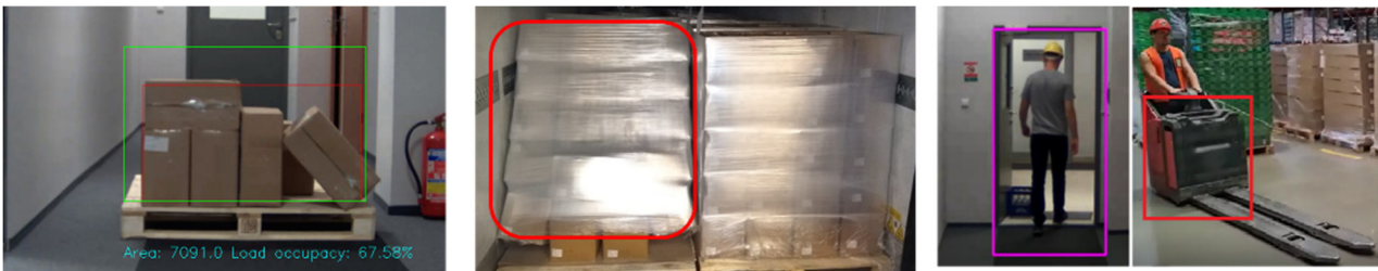
Figure 1 Optidata object detection applications (from left: load occupancy estimation, unit load defect detection, real-time object detection)
