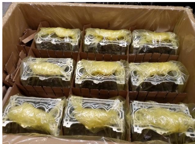
Figure 1 Cylinder blocks for 1.5 I TSI engines prepared for expedition to Mexico
