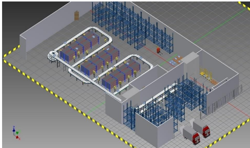
Figure 1 The current 3D layout of the main (left) and shipping warehouse (right)
