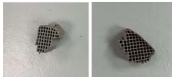
Figure 2 Pieces from catalyst number 1 [6]
