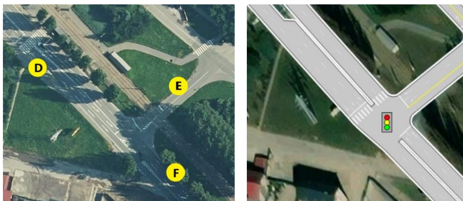
Figure 5 Model of the original state (left) and the proposed state of the Dneperská intersection with traffic lights (right)
