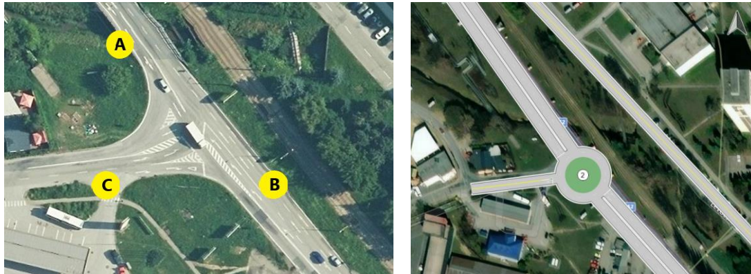
Figure 4 The original state (left) and the proposed state of the intersection Textilná (right)
