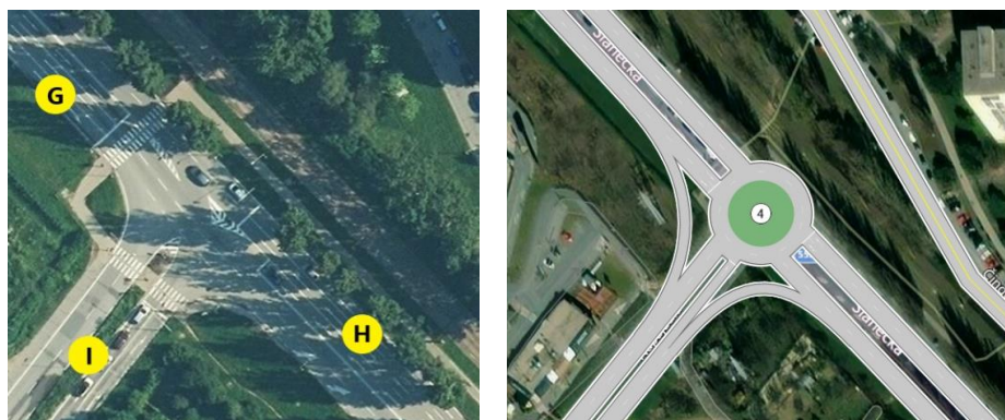
Figure 6 Model of the original state (left) and the proposed state of the Napájadla intersection (right)
